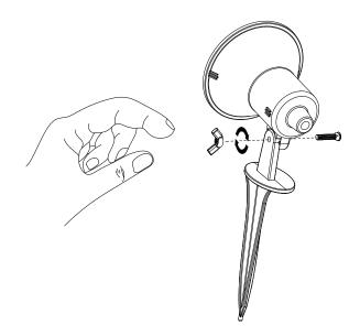
**Option 2:** To attach the wall mount base, use the included screw and washer. Align the hole on the stake to the hole on the flood light housing. Slide the screw through the hole and turn the fastener clockwise until tight. (This option requires extra screws to be installed onto the wall/siding of your choice. A power drill is required for this option.)
